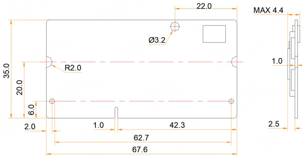
Tolerance:  $\pm 0.3$  Unit: mm
