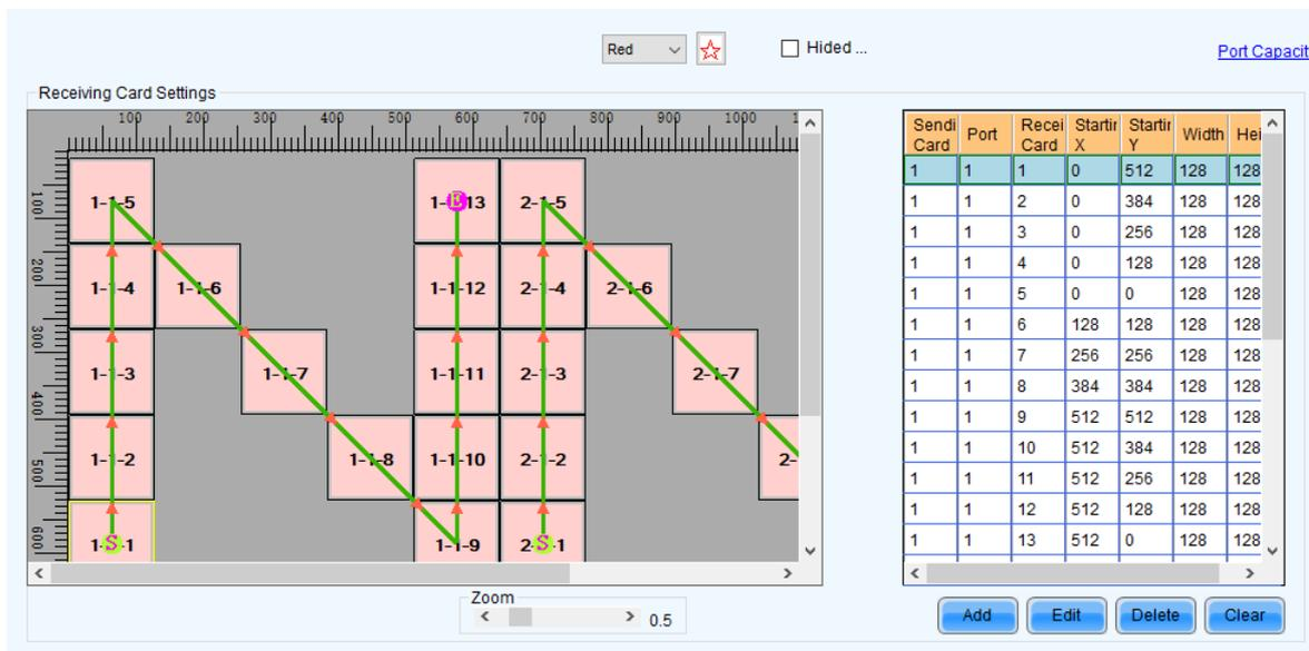
Step 8 Click **Send to HW** to send the configuration information to the hardware. If necessary, click **Save to File** to save the configuration information as a file.
