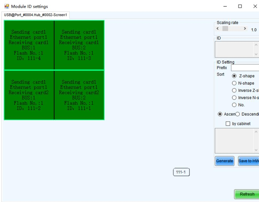
Figure 8-8 Setting module ID (complex screen)
