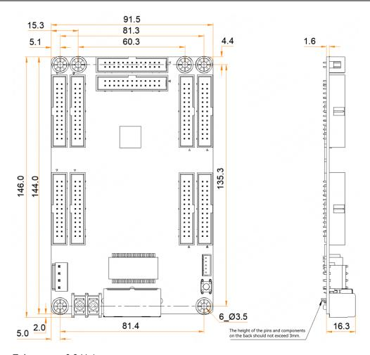
Tolerance: ±0.3 Unit: mm
