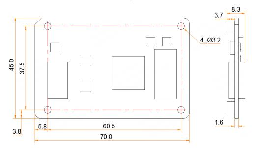
Tolerance: ±0.3 Unit: mm
