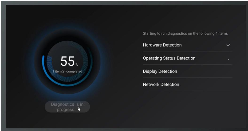
Step 3 Once the diagnostic process is complete, you will see either **Device normal** or **Device abnormal** displayed on the left. On the right, you can view the test items categorized as **Normal**, **Abnormal**, or **Not tested**. To see detailed information about all detected items, select **View Report**.
