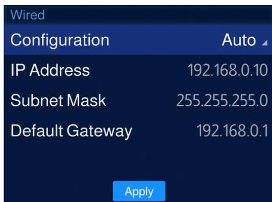
Step 3 If **Manual** is selected, specify a correct **IP Address**, **Subnet Mask**, **Default Gateway** and **DNS**, then select **Apply**. If **Auto** is selected, this step is not required.
