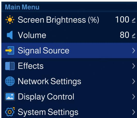
Step 2 Select a signal source (Android, HDMI 1, HDMI 2 or HDMI 3). Press the knob after a signal source is selected.
