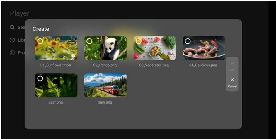
Step 4 After selecting a program, long press the **Confirm** button on the remote to access options such as renaming, batch selection, and deletion (The default program cannot be edited).
