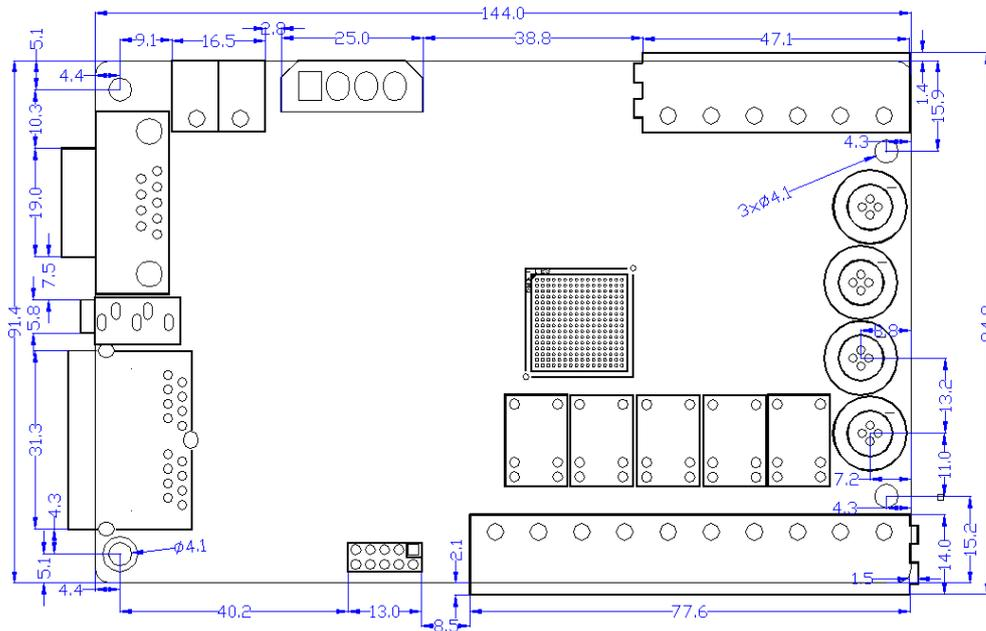
Tolerance: ±0.3 Unit: mm
