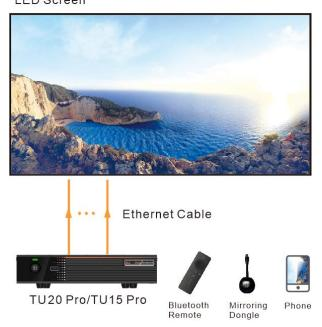
Step 4 Connect the Ethernet cables from the LED screen to the Ethernet output ports of TU20 Pro/TU15 Pro in the order shown below.
