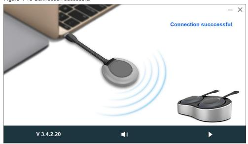
Step 3 When a pop-up window with the "Connection successful" message appears on the desktop, press the round button on the dongle to start mirroring.
