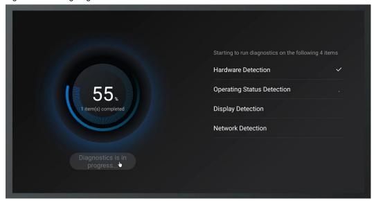
Once the diagnostic process is complete, you will see either Device normal or Device abnormal Step 3 displayed on the left. On the right, you can view the test items categorized as Normal, Abnormal, or Not tested. To see detailed information about all detected items, click View Report.
