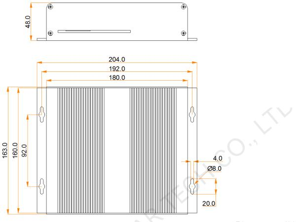
Tolerance: ±0.3 Unit: mm
