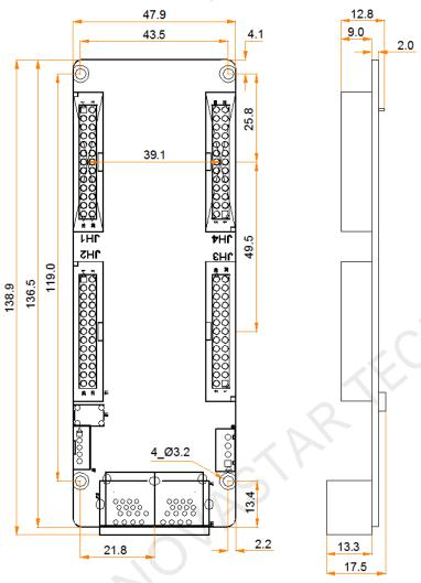
Tolerance: ±0.1 Unit: mm
